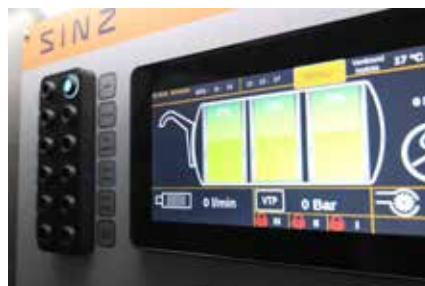
Detail of the touch screen with resolution 1280x480px.
